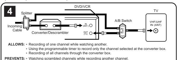
DVD/VCR TV Splitter VHF/UHF ∄→ (ANT.) O IN (ANT) A/B Switch Converter/ Incoming Descrambler Cable **ALLOWS:** \* Recording of nonscrambled channels. \* Recording of one channel while watching another. \* Watching premium channels through the converter while recording nonscrambled channels. \* Using the programmable timer. PREVENTS: Recording scrambled channels.
